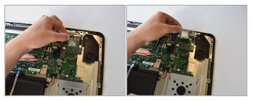
• Remove the wireless card from the casing by lifting up then pulling out.
