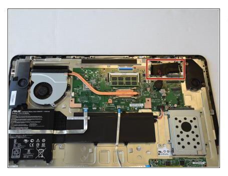
The wireless card is on the corner of the motherboard next to the speaker. Remove the black tape to reveal the wireless card.
