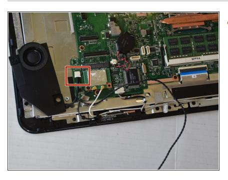
Pull the cord attached to the speaker out of the motherboard
