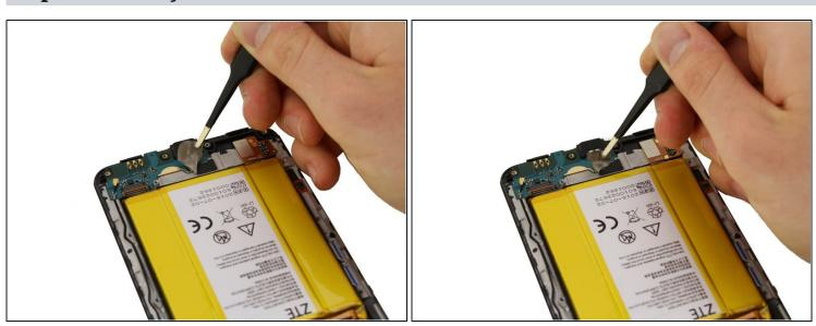
• Use <u>tweezers</u> to peel off the tape at the bottom of the phone.
