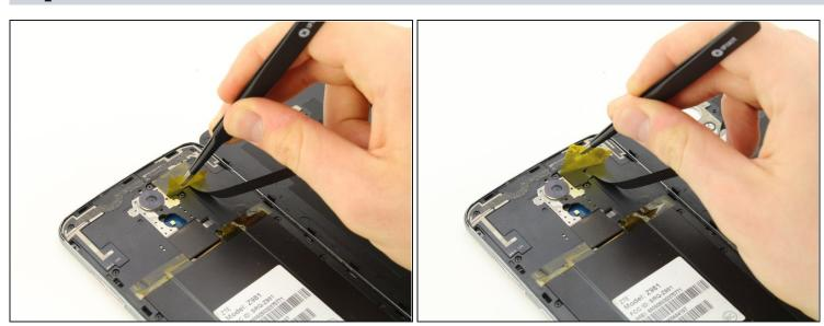
• Remove the yellow Kapton tape by using the <u>tweezers</u> to peel it up and away from the device.
