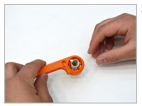
• Put the spring into the replacement brake handle.
