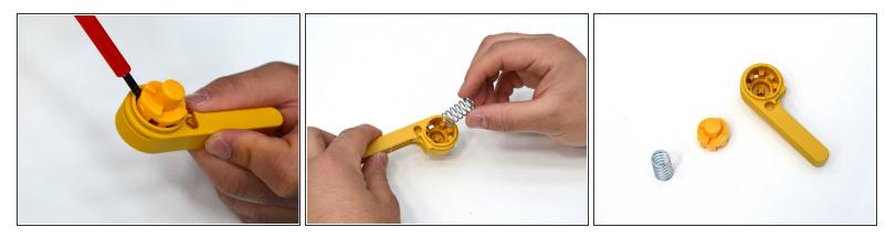
• Pry the inside part out of the brake with a flat screwdriver.
