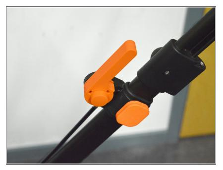
Insert the brake handle back into the frame.
