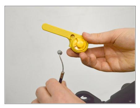
• Take the brake cable out of the groove in the brake handle.
