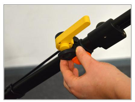
• Remove the left piece that is holding the brake handle.
