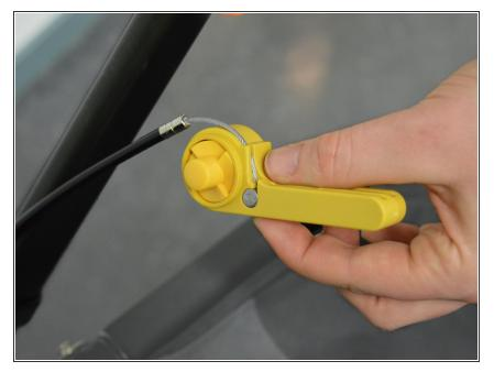
• Pull the brake line down and take the brake handle out of the black plastic part.
