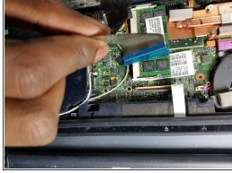
There will be a metallic film attached to the keyboard from the motherboard. A black latch runs along the film keeping it in place. Lift the latch and detach the film; remove it to fully remove the keyboard.
