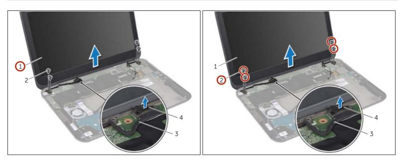
Place the NEW display assembly in position and replace the screws that secure the display assembly to the computer base.
