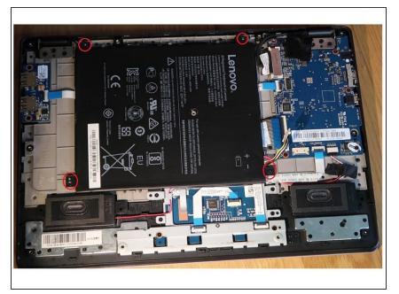
Next remove the four screws holding the battery in place.
