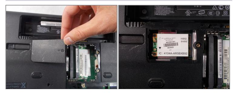
• Lift up on the screw side to remove the panel.
