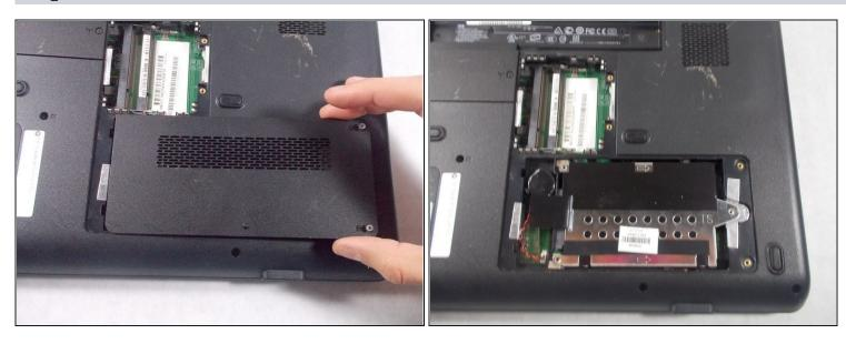
• After the screws are removed, slide the hard drive panel to right to remove it.
