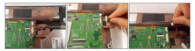
• Using a spudger, remove both additional highlighted wires from the motherboad.
