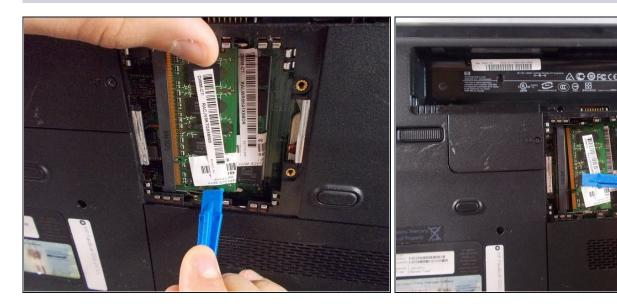
• Gently pull apart the two metal tabs located on both sides of the stick of RAM.
