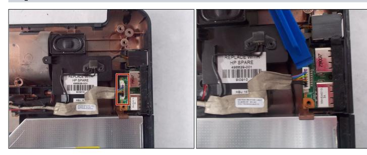
• Using a spudger, remove the highlighted white wire.
