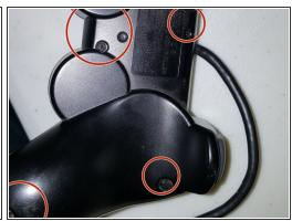
• There are 6 screws that you will want to remove on the back of the Dualshock 2 controller. All pictures show the same thing essentially, but because of Ifixit's odd picture cropping system, every screw appears at least once throughout the 3 photos.
