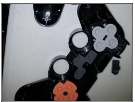
• The casing should come right off, followed by the circuit board, the the white-plastic part. Make sure to keep track of all your buttons, as when you are taking it apart, they can be lost easily.
