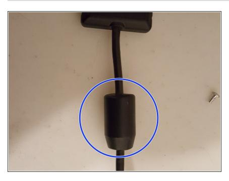
• How it works" This little plastic bulge is actually just a piece of magnetized ferrite. What it does is allow for reduce electrical interference and thereby enable more efficient flow of electrons or electrical current to and from the device.
