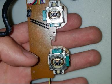
• In the first picture, you can see the bottom of the top shell of the Dualshock 2 controller. In the second one, you can see the joysticks without the rubber part.
