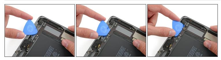
Slide an opening pick under the logic board from the front-facing camera to the rear facing camera.
