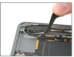
• Carefully peel the LCD buffer tape up off of the rear case.
