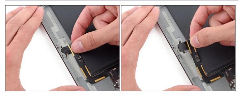
• Pull the Lightning connector straight out of its recess in the rear case.
