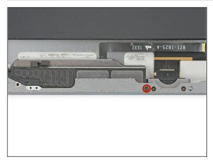
• Remove the 2.2 mm Phillips #000 screw securing the speaker to the rear case.
