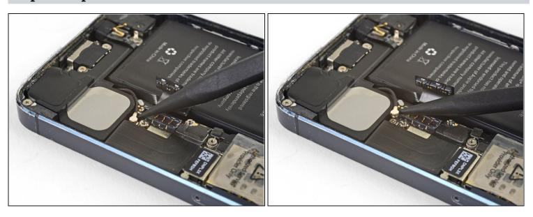
• Use the point of a spudger to pry up and disconnect the antenna cable from the logic board.
