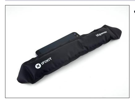
Flip the phone face up, <u>heat an</u> <u>iOpener</u>, and apply it to the right edge of the phone for a minute.
