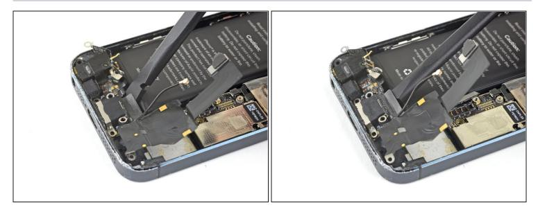
• Use the flat end of a spudger to loosen the rest of the Lightning connector assembly from the rear case.
