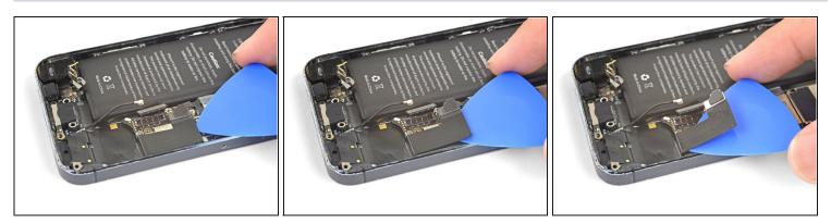
• Slide an opening pick underneath the Lightning connector flex cable to loosen it from the logic board and the rear case.
