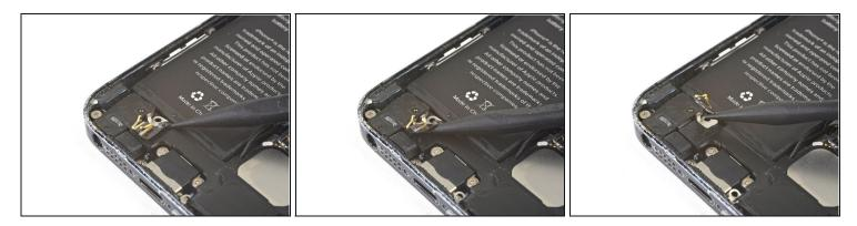
• Slide the point of a spudger underneath the spring contact flex cable below the battery and gently loosen it from the speaker enclosure.
