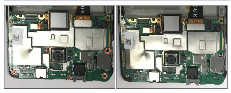
• Remove the five 1.5mm Phillips #000 screws from the motherboard.
