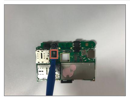
Use a plastic opening tool to pry the front camera connector from its socket on the motherboard.
