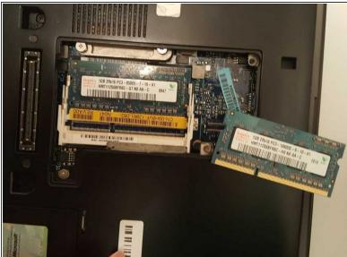
Slide the RAM backwards out of its socket to remove.
