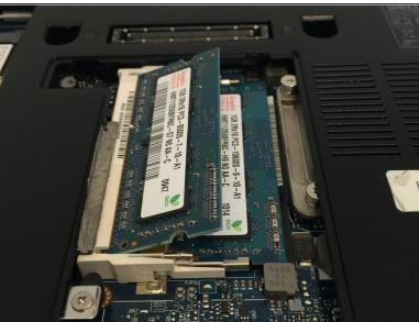
Pry the two metal clips away from the RAM module until the module pops out of place.
