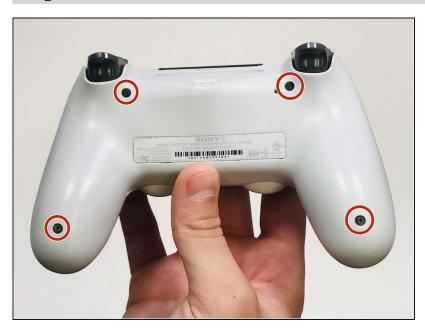
Remove the four 2mm screws on the rear plate using the #000 Phillips screwdriver.
