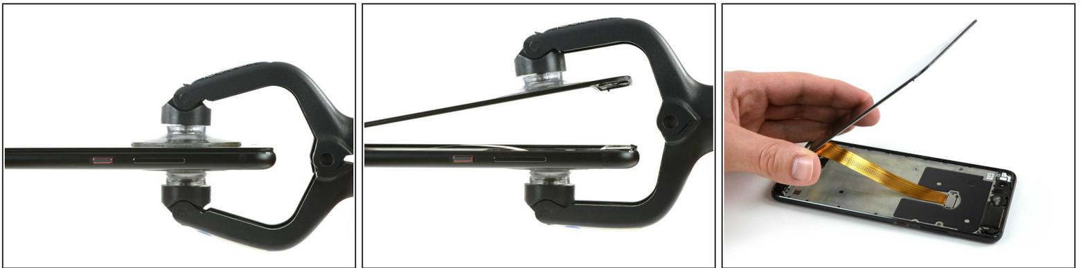
**⚠ There is a thin display cable between the screen and phone, be very careful not to rip it when opening the device.**
