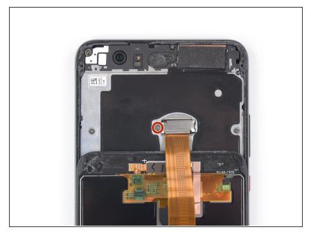
Remove the 3.3 mm-long Phillips screw securing the display flex connector bracket.
