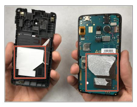
After the clips are released, carefully separate the back housing from the phone. Notice the sticker that appears in the red box holds the phone together, but can be peeled apart.
