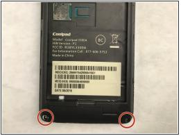
Remove the four screws (30 mm long) which hold the front and back half of the unit together using a Phillips #000 screwdriver. There will be one screw in each corner.
