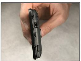
Use a metal spudger to release all of the clips around the phone. These clips are used to hold the front and back panel on the phone together.
