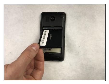
After removing the back of the phone (not pictured), remove the battery by lifting up from the bottom with your thumb. There will be a groove that allows you to remove the battery with your thumb.
