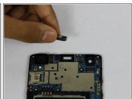
Using a plastic opening tool, pry up the front facing speaker and remove it from the phone.
