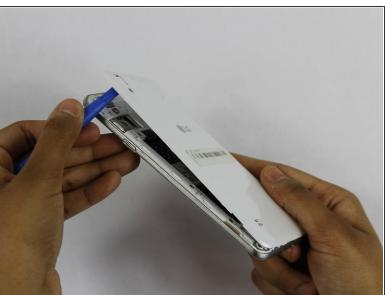
Insert a fingernail, or plastic opening tool, into the cutout on the back cover and pry outward to remove.
