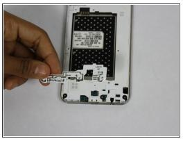
• Using a plastic opening tool, remove the antenna extender from the bottom.
