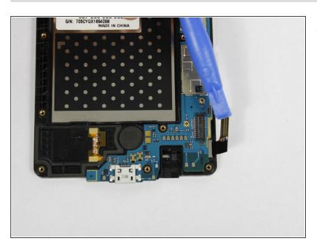
Disconnect the LCD from the motherboard with a plastic opening tool.
