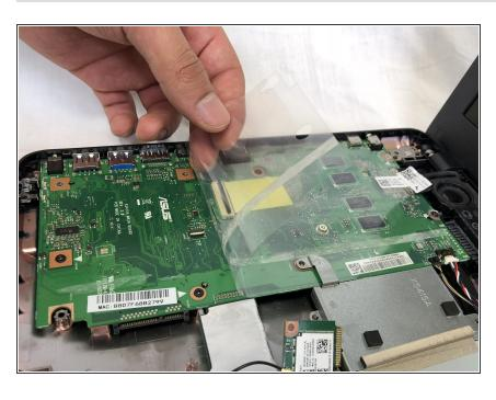
Remove the plastic covering off of the motherboard.
