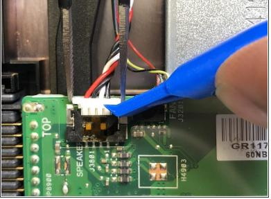
Remove the cables connected to the motherboard by unplugging them using a plastic opening tool, or by hand.
