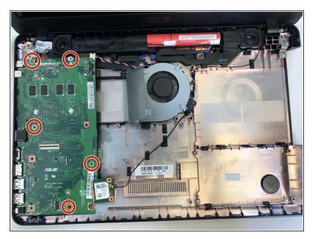
Remove the five 6mm Phillips #0 screws from the motherboard.
