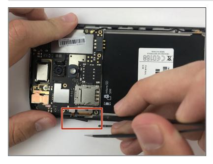
Remove the power button by pushing the round tip out using the tweezers (or a pen if you don't have tweezers).
