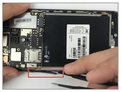
Remove the volume button by pushing the round tips out using the <u>tweezers</u> (or a pen if you don't have tweezers).
