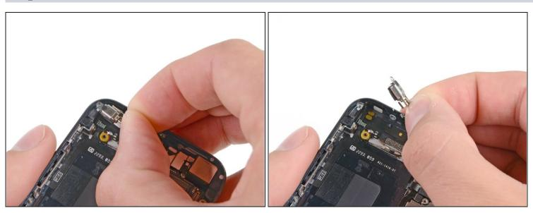
• Remove the vibrator from the rear case.
