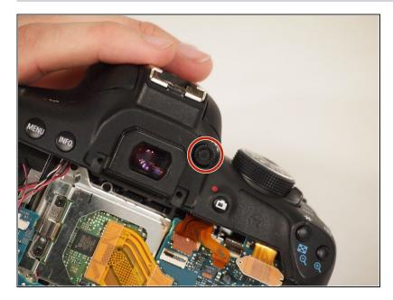
Remove the diopter adjustment knob next to the viewfinder using a JIS #000 screwdriver.
