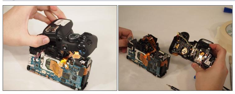
• Remove the entire upper flash assembly by gently pulling it up and off the camera.
