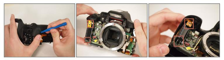
• Using the plastic opening tool, pry the front of the casing off of the camera.
