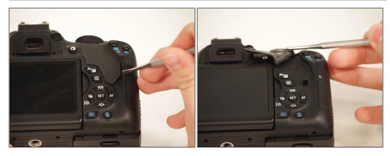
• Using the metal spudger, pry the rubber grip located just below the turndial.
