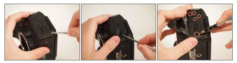
• Using a metal spudger, pry the rubber grip off of the casing on the left side of the camera.
