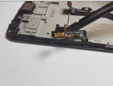
• Use the <u>Plastic Spudger</u> to finish lifting the volume and power buttons flex from the base of the phone.
