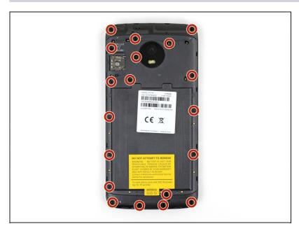
Remove the nineteen 3.2 mm long T3 screws securing the plastic midframe.
