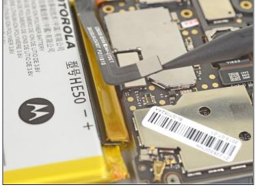
• Use the point of a spudger to pry up and disconnect the battery connector from its motherboard socket.
