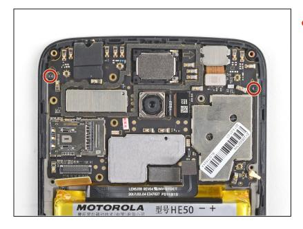
• Remove the two black 3.2 mm long T3 screws securing the motherboard.
