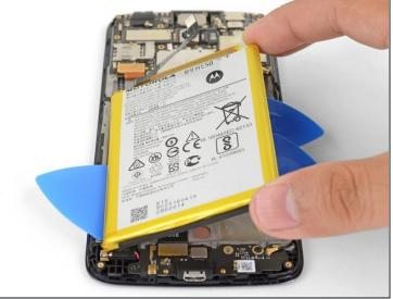
Grasp the battery along the right corners and slowly lift the right edge upwards.
