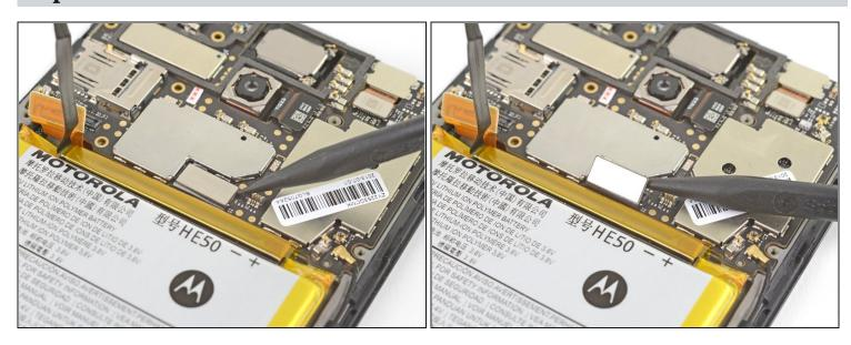
• Use the point of a spudger to pry up and disconnect the interconnect cable from its motherboard socket.
