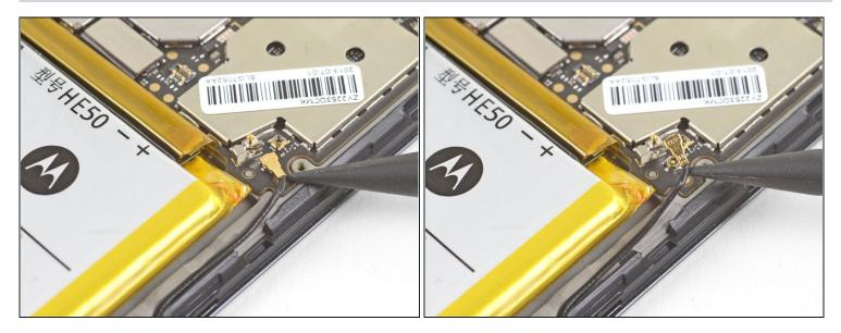
• Use the point of a spudger to pry up and disconnect the antenna cable from its motherboard socket.
