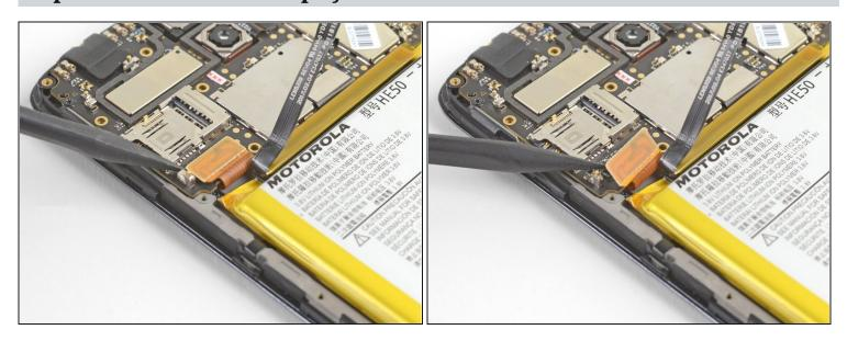
• Use the point of a spudger to pry up and disconnect the display cable from its motherboard socket, near the bottom left corner of the motherboard.
