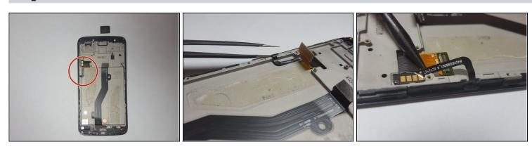
• Use the <u>Precision Tweezer</u> to detach the <u>Power and Volume Buttons Flex</u>. Start at the lip of the phone, as seen in Image 2, and lift up. Slide the precision <u>tweezers</u> under the power and volume buttons flex until you reach the gold plated section, detaching it from the phone.
