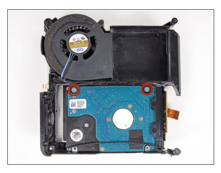
Remove the two Phillips screws connecting the underside of the hard drive to the internal frame.
