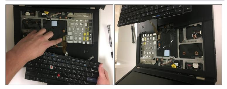
• Slide the keyboard out of the way until you can see what's underneath it.
