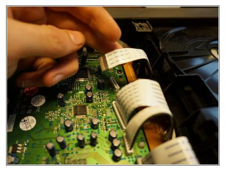
Remove all ribbons with great care gently wiggling side to side while applying force perpendicular to the circuit board
