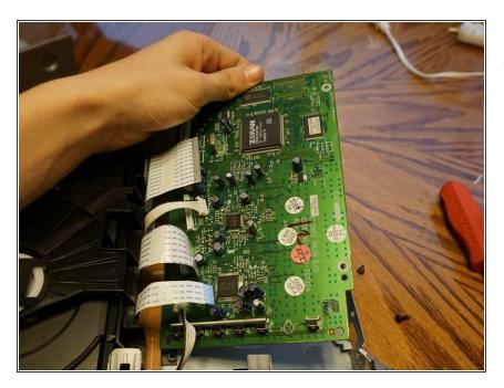
Gently tilt up the board making sure to check the ribbon connections twice
