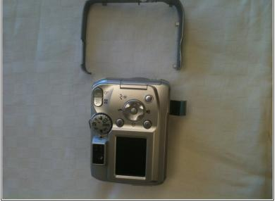
Locate the gray band that you removed the screws from; this holds the two halves of the camera together. Use an iPod fix-it tool to pry the gray band loose and remove it.
