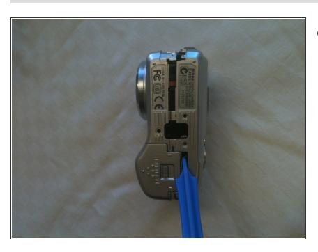
Use the iPod fix-it tool to separate the back panel from the camera.
