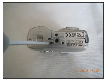
Locate the 3 black screws on the bottom of the camera and the 2 gray screws on each side of the camera.
