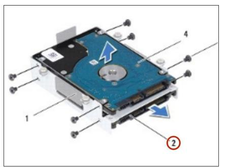
• If applicable, slide the secondary hard drive into the hard-drive bracket.
