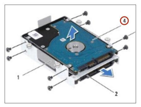
Place the primary hard drive (HDD0) in the hard-drive bracket.
