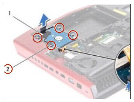
• Tighten the four captive screws that secure the hard-drive assembly to the computer base.
