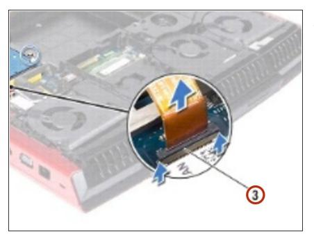
Connect the hard-drive cable to the connector on the system board and press down on the connector latch to secure the cable.
