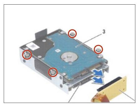
• Replace the four screws that secure the primary hard drive (HDD 0).
