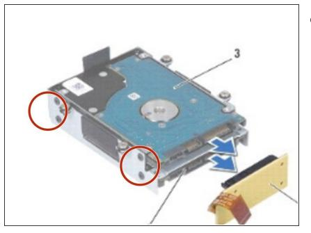
Remove the four screws that secure the primary hard drive (HDD 0) and lift the hard drive out of the hard drive bracket.
