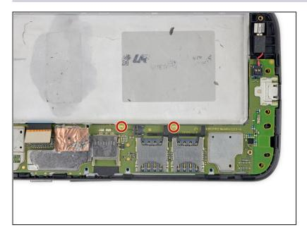
Use a T3 Torx driver to remove the two bronze-colored, 2.4 mm screws securing the motherboard.
