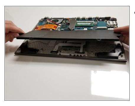
Lift the battery up by its sides. The battery should easily come off.
