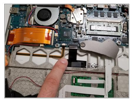
Locate two <u>ZIF (Zero Insert Force)</u> connector cables underneath the battery.
