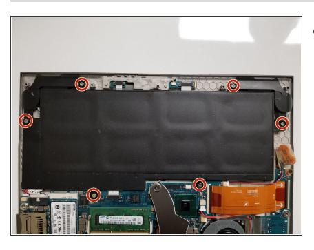
Remove the six screws using a Phillips #1 screwdriver.
