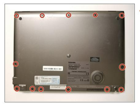
Remove the thirteen 1.4mm screws using a Phillips #2 screwdriver
