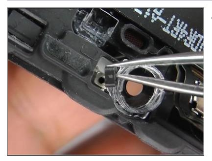
There is a small, black plastic spacer underneath the metal bracket at the upper screw. The upper screw goes through the metal bracket then through this plastic spacer.
