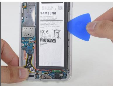
Slide the opening pick up the side of the battery to break apart any remaining adhesive.
