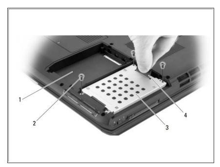
Using the pull-tab on the hard drive, pull the hard drive out of the hard drive bay.
