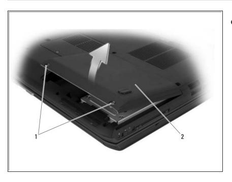
Loosen the two captive screws and remove the hard-drive bay cover.
