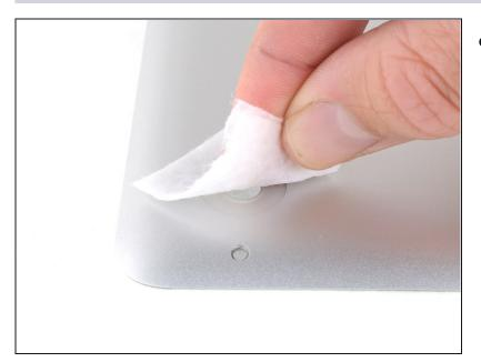
• Scrub the foot pad with adhesive remover to remove any remaining adhesive.
