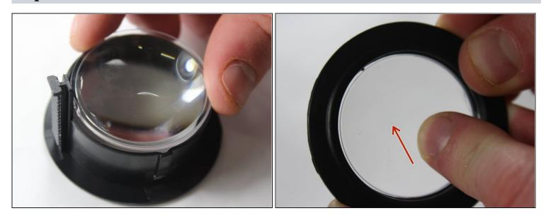
• To get the actual lens out, you will need to push the lens from the outside in with a little force to break the lens out of it's case.
