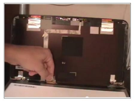
• Place the new screen on the keyboard and connect cable
