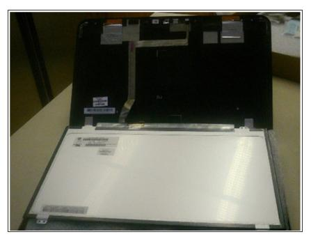
• Remove screen from back panel and lay it on the keyboard
