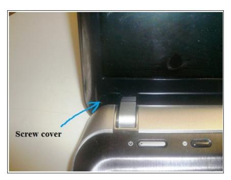
Remove screw covers in both sides with the knife
