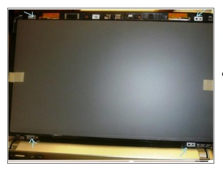
Place the screen into the back cover and install 4 screws. Install the bezel, battery, and then turn on computer ENJOY WITH YOUR NEW SCREEN. Go to website link at below to order the new screen http://www.laptopscreen.com/English /mode...
