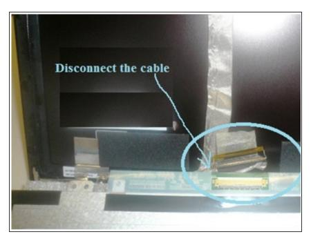
• Use the tweezer to remove the tape and then disconnect the cable
