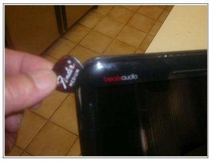
Use guitar pick to unclip the screen bezel
