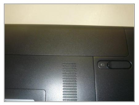
• Turn off computer and remove the battery in the back side
