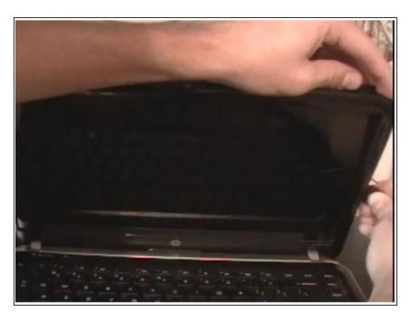
Use guitar pick to unclip the screen bezel
