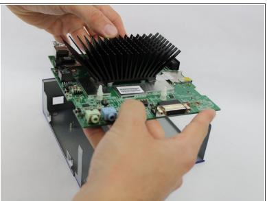
Lift the motherboard out of the casing.
