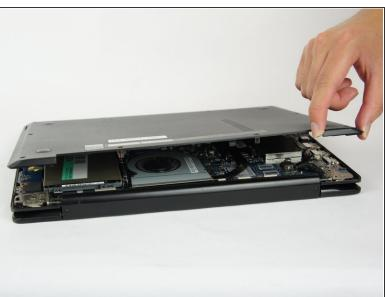
Pry open the back casing using the opening tool along the side crevice.
