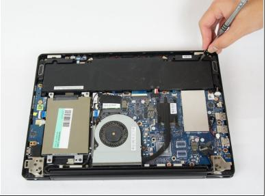
Using the JIS #0 Screwdriver, remove the five 5.0 mm screws that hold down the battery.
