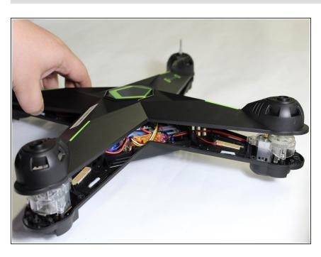
Separate the upper and lower housing units by lightly pulling the two housing units apart.
