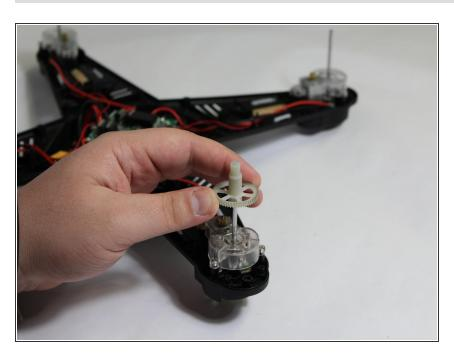
Lift the pinion gear off the motor shaft by lightly pulling it away from the drone.
