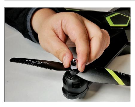
Remove the chrome shaft cover by lightly pulling it away from the drone.
