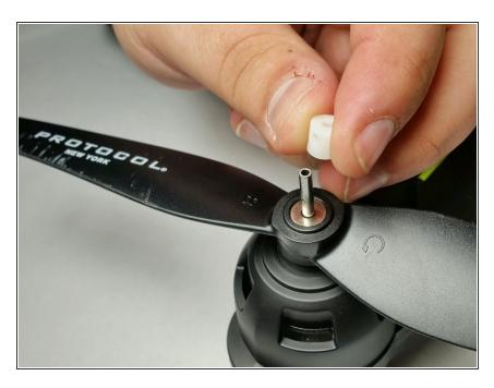
Remove the propeller stop from shaft by lightly pulling it away from the drone.
