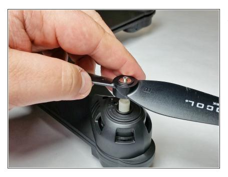
Remove the propeller from shaft by lightly pulling it away from the drone.
