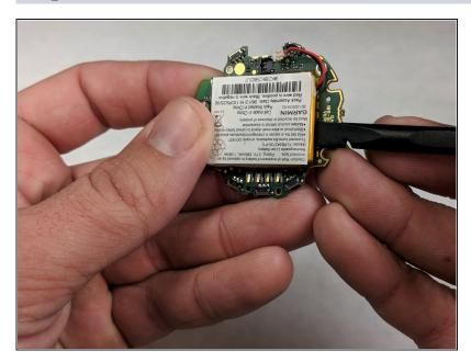
The battery is glued to the motherboard and will need pried off using the nylon spudger.
