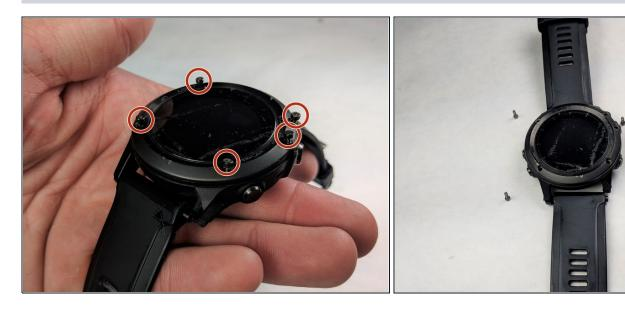
• Remove the five 7mm screws with H1.3 hex screwdriver.
