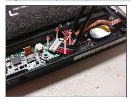
To remove the battery, take some tweezers or a spudger and carefully pop the connector off vertically; it looks like it might come out perpendicular to the board, but it comes straight off with some gentle prying from underneath.
