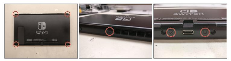
• Using the Y1 Screwdriver, remove the four tri-point screws on the back of the device, in the corners; then a single screw on top, and two screws on either side of the charging port.
