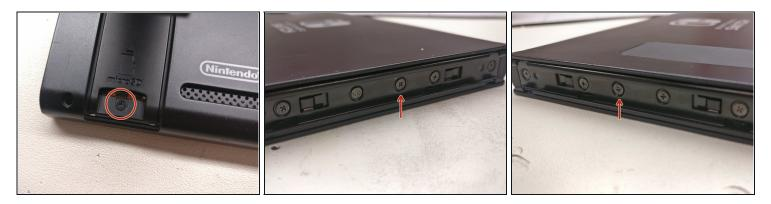
• Be sure to lift up the kickstand and remove this sneaky little screw around the SD card slot, and then the center screws on both sides of the device, where the Joycon brackets are screwed in place.
