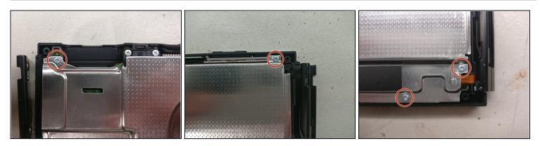
• Remove the circled screws on the back of the metal plate, as indicated by the photos, but don't attempt to pull it off yet.
