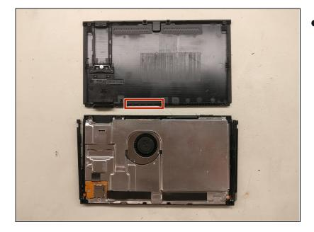
With the myriad of screws removed, you should now be able to pop the back cover off with minimal prying; you might need an iSesamo style spudger to get it started , just make sure you're careful around the fan exhaust, (marked in the photo) there's some tiny clips that you wouldn't want to pull off with too much force.
