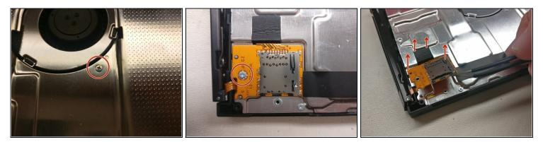
• Take out the center screw, near the blower fan, and the screw in the small SD card reader assembly. Then using <u>tweezers</u> or a spudger, carefully remove the SD card reader and detach the flex cable from the board; you can do this by carefully sliding a spudger under the area covered by the foam and gently prying up. it comes off fairly easily.
