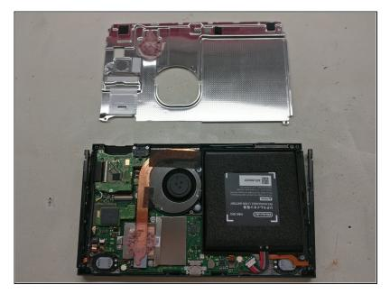
• You can now gently pull the metal plate off and set it aside, revealing the tightly designed internals of the switch, along with your battery.
