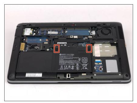
Unlatch the two latches securing the battery in the case.
