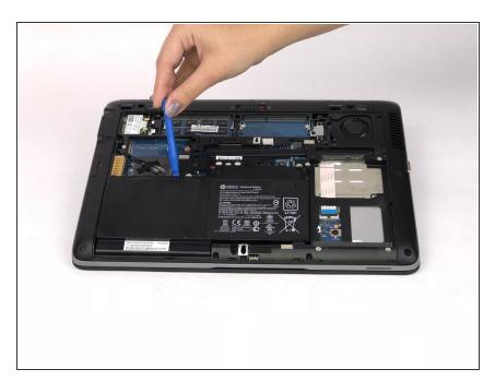
Use a plastic opening tool to lift and remove the battery.
