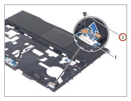
Remove the screw that secures the status-light board to the palm-rest assembly.
