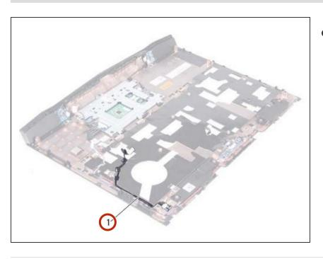
Route the status-light board cable through the routing guides on the palm-rest assembly.
