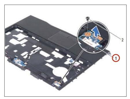
Carefully lift the status-light board and release its cable from the slot on the palm-rest assembly.
