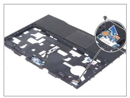
Align the slot on the status-light board with the alignment post on the palm-rest assembly.
