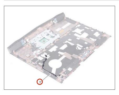
Slide the **NEW** status-light board cable through the slot in the palmrest assembly.
