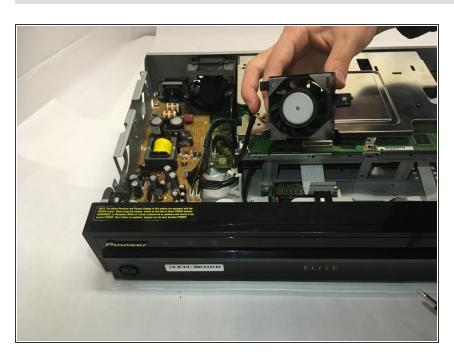
Grip the frame of the cooling fan and slide it toward the front panel, then lift out of the device.
