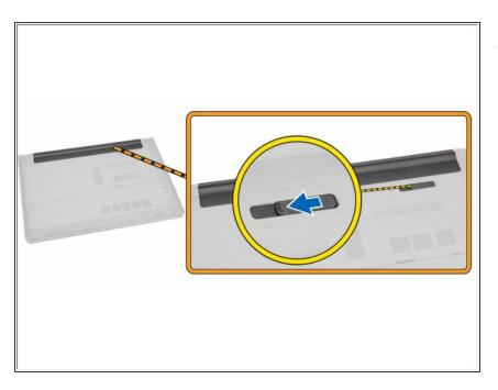
• Slide the release latch outwards to unlock the battery.
