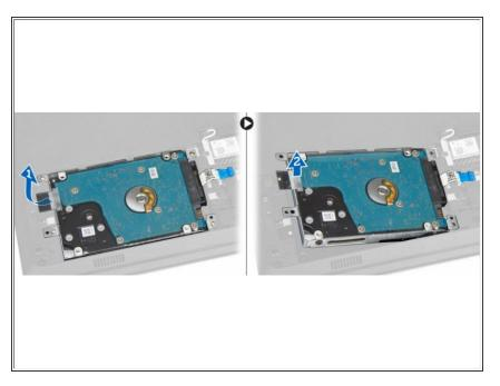
Remove the tape and lift the hard drive to remove it from the computer.
