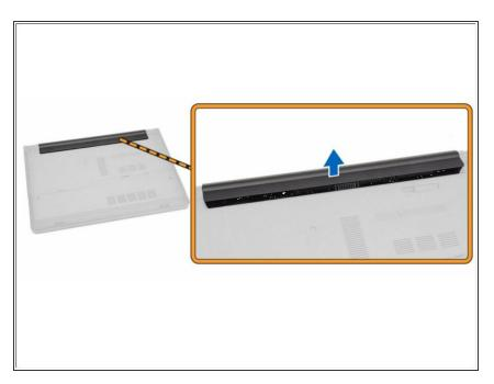
• Lift the battery to remove it from the computer.
