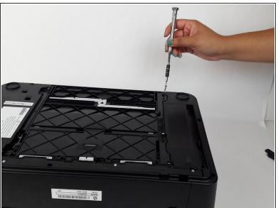
Locate and remove the farthest 13mm TR10 Torx Security screw.
