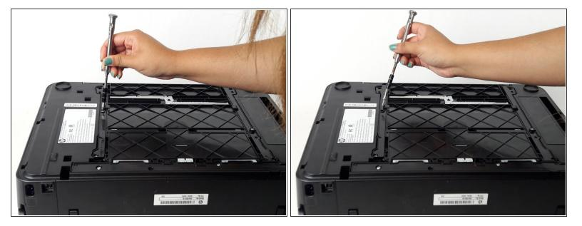
Locate and remove middle 13mm TR10 Torx Security screw using a Torx screwdriver.
