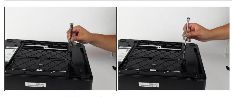
Locate middle 13mm TR10 Torx Security screw and remove it.
