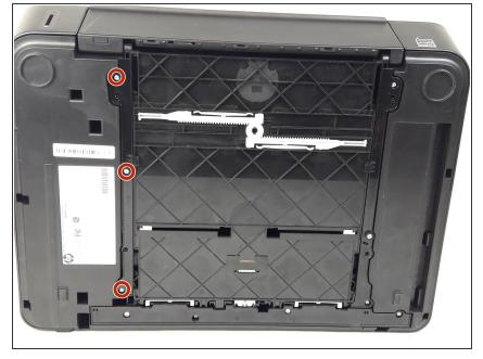
Locate the 13mm TR10 Torx screws on the left side of the paper tray.
