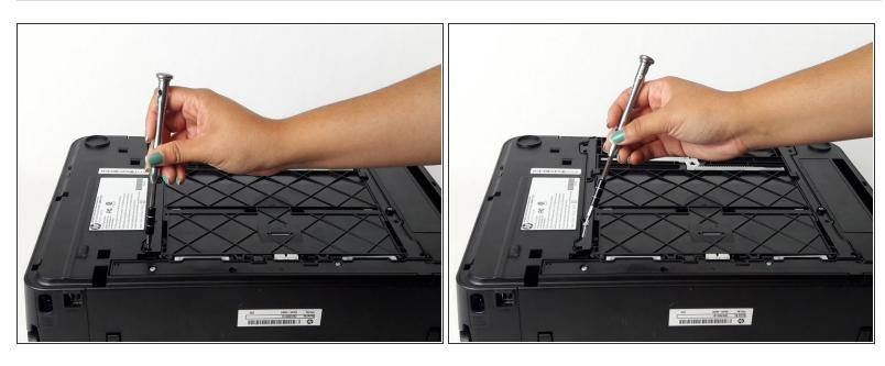
Locate and remove the last 13mm TR10 Torx Security screw.
