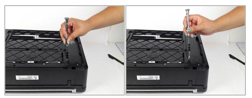
Locate last 13mm TR10 Torx Security screw and remove it.
