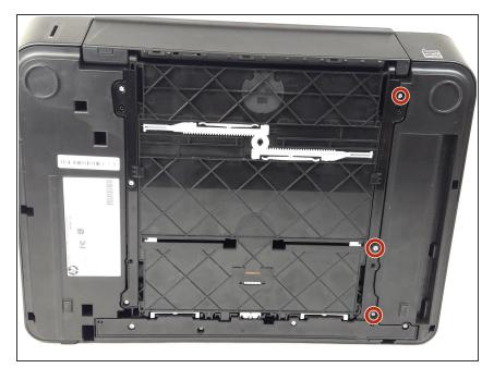
Locate the three 13mm TR10 Torx Security screws on the right side panel.
