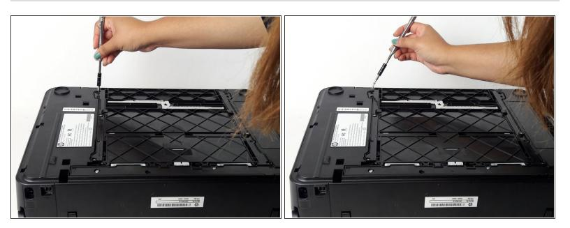
Unscrew and remove the 13mm TR10 Torx Security screw, starting with the farthest screw on the left
