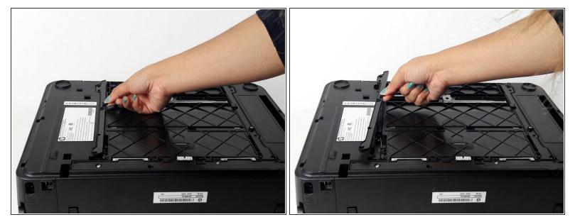
Locate the side tab and lift up to remove.
