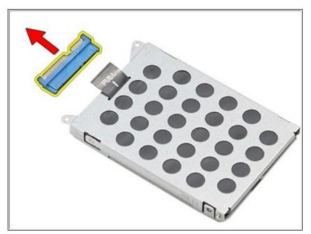
• Remove the hard-drive adapter from the hard-drive assembly.
