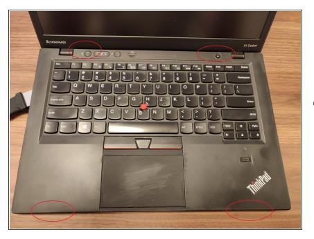
Turn the laptop right side up, and open the screen. Slide the plastic the spudger along the edge of the
