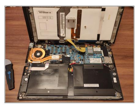
• Gently lift the keyboard away from you, as you would open the screen. The cable connecting the keyboard to the chassis is at the top. It will want to shift slightly to the right as you open it to account for the cable.
