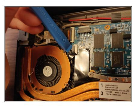
Gently lift the CPU fan cable socket latch, and pull the cable to the left to remove.
