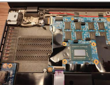
• Clean the CPU with isopropyl alcohol, and the dust catcher for any debris/dust.
