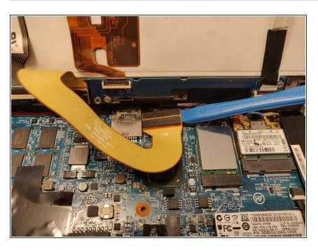
Gently pry away the keyboard connector from the chassis, and set the keyboard aside.
