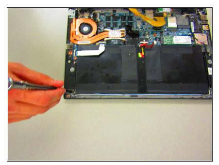
Unscrew the 4 screws holding the battery in place.
