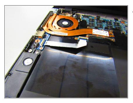
Unlock and remove the ribbon cable running over the top of the battery.
