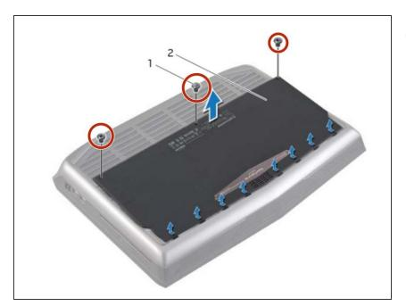
Use a Phillips screwdriver to remove the three screws securing the base cover.
